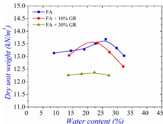
Fig. 5. Compaction curve for FA-GR mixtures under Standard Proctor energy
