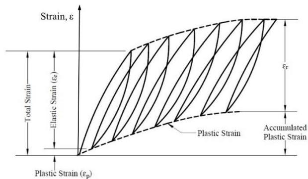
**Fig. 1.** Variation of strain for the repeated load application (modified after Huang 2004).
