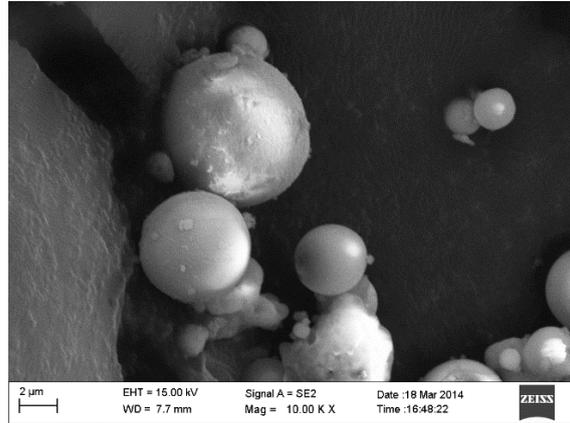
**Fig. 4.** SEM image of FA at 10,000 X magnification
