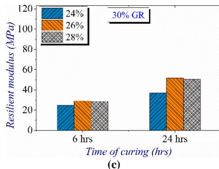
**Fig. 7.** Resilient modulus values corresponding to different cases at different water contents and after 6- and 24-hours curing periods (a) 0% GR (only FA), (b) FA+10% GR and (c) FA+30% GR
