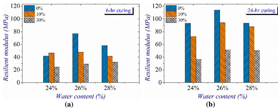
**Fig. 8.** Resilient modulus vs. water content at curing periods of (a) 6 hours and (b) 24 hours
