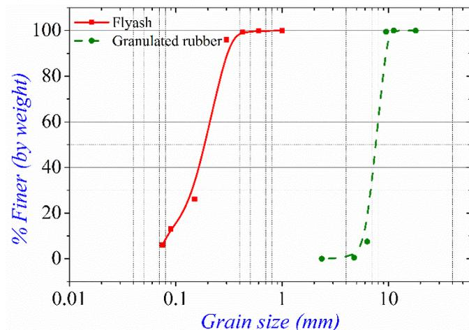
Fig. 3. Particle size distribution of FA and GR
