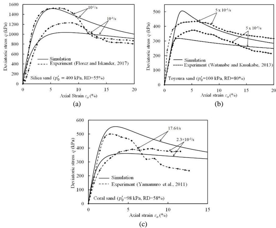
**Fig. 1** Evolution of stress-strain response for (a) silica sand (b) Toyoura sand and (c) coral sand subjected to rate-dependent drained triaxial condition with varying strain rate.
