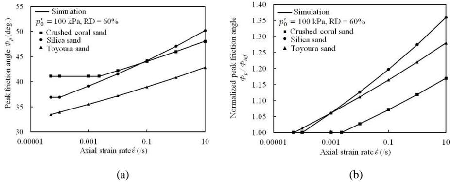
**Fig. 3** Variation in the (a) peak friction angle ( $\Phi_p$ ) and (b) normalized friction angle ( $\Phi_p/\Phi_{p,ref}$ ) for different sand types over the selected strain rate range when subjected to drained triaxial condition at initial confinement  $p'_0 = 100$  kPa and relative density  $RD = 60\%$ .
