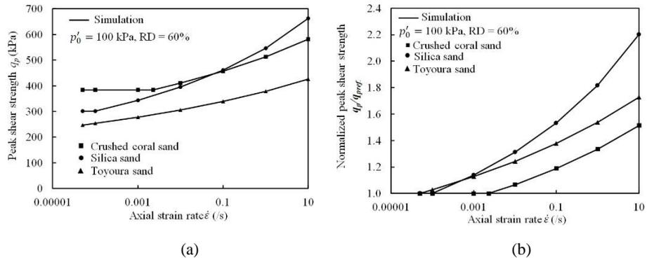
**Fig. 2** Variation in the (a) peak shear strength ( $q_p$ ) and (b) normalized peak shear strength ( $q_p/q_{p,ref}$ ) for different sand types over the selected strain rate range when subjected to drained triaxial condition at initial confinement  $p'_0 = 100$  kPa and relative density  $RD = 60\%$ .
