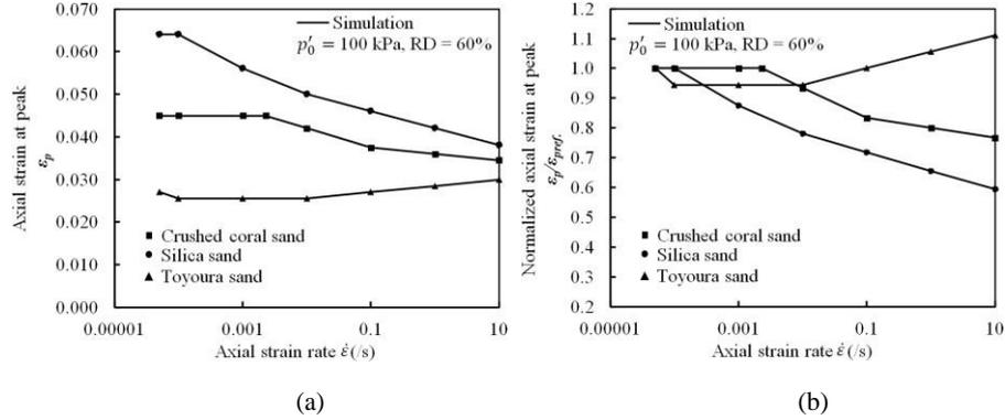
**Fig. 4** Variation in the (a) axial strain at peak ( $\epsilon_p$ ) and (b) normalized axial strain at peak ( $\epsilon_p/\epsilon_{p,ref}$ ) for different sand types over the selected strain rate range when subjected to drained triaxial condition at initial confinement  $p'_0 = 100$  kPa and relative density  $RD = 60\%$ .
