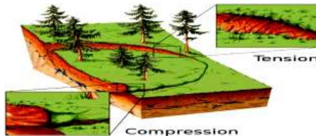
**Fig. 2.** Loading of roots under tension and compression depending on their position (lateral or at the toe of the slope) during the triggering of a shallow landslide. The unstable soil mass pushes down, creating passive earth pressure conditions in the down slope edge (after Baum et al., 2008).
