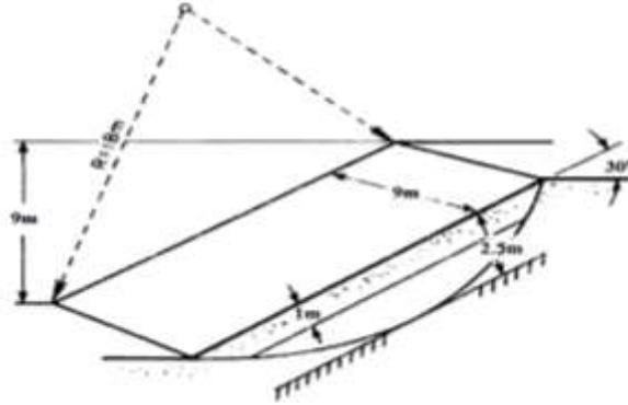
**Fig. 9.** Stability and Analysis of Three Dimensional Slip Surface (after Wu, 1984)
