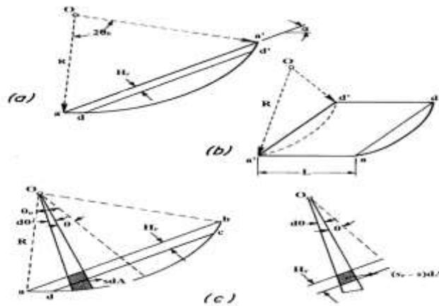
Fig. 8. Three Dimensional Slip Surface: (a) Side View, (b) Perspective View and, (c) Computing of resisting moment (after Wu, 1984)
