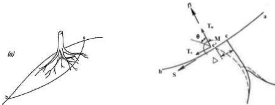
**Fig. 5.** Soil reinforcement by root (a) intersection of root with slip surface (b) forces on root and root displacement (after Wu, 1984)
