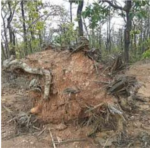
**Fig. 6.** Intersection of roots with the ends of cylindrical slip surface
