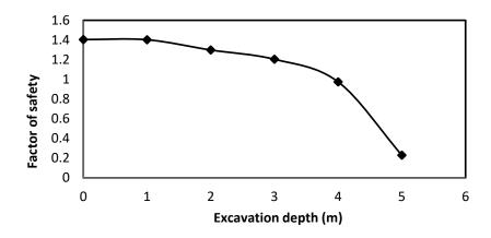
Fig. 2. Variation of factor of safety with excavation depth
