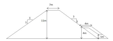
Fig. 6. Remediated section for existing portion of dam
