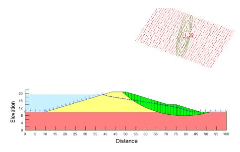
Fig. 5. Stability analysis of existing section with berm height 4m
