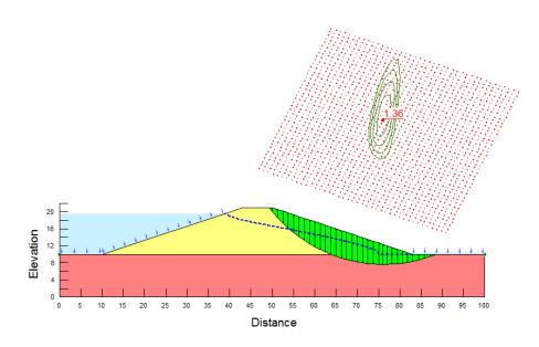
Fig. 1. Slope stability analysis of failed section under steady state seepage using GeoStudio
