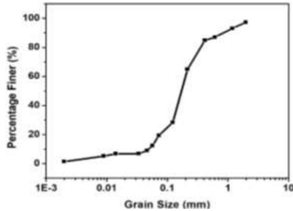
Fig. 1. Grain size distribution of Fly ash
