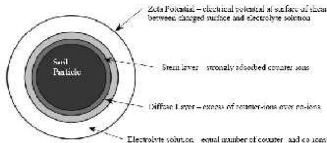
Fig. 2.2 Idealized Representation of Water Around A Clay Particle
