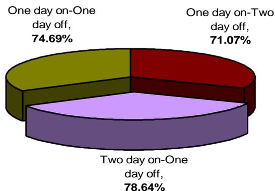
Fig. 12 Total Percentage Removal Of Nickel After Electrokinetic Remediation
