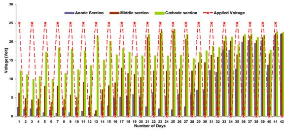
Fig. 2 Variation Of Voltage At Different Sections Along Length Of Sample & Applied Voltage With Time for one day on and one day off model
