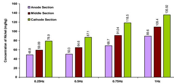
Fig 21 Concentration Of Metal After Electrokinetic Remediation
