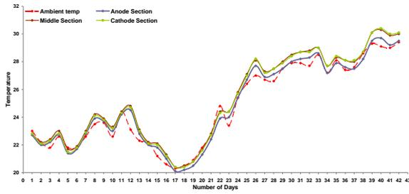
Fig. 17 Variation Of Temperature & Ambient Temperature With Time for 0.75 Hz Frequency
