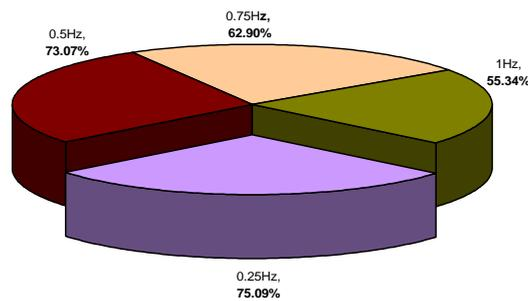
Fig 22 Total Percentage removal of Nickel After Electrokinetics Remediation Using Low Frequency AC Supply
