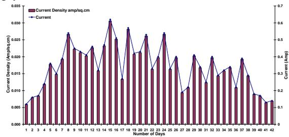
Fig. 9 Variation Of Current And Current Density With Respect To Time for Two days on and One day Off model
