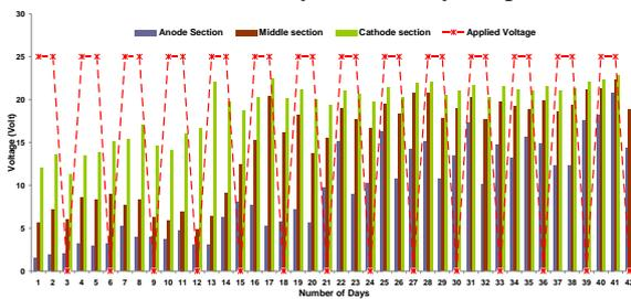
Fig. 8 Variation Of Voltage At Different Sections Along Length Of Sample & Applied Voltage With Time for Two days on and One day Off model
