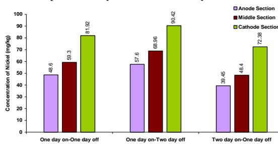
Fig. 11 Concentration Of Metal After Electrokinetic Remediation
