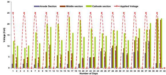
Fig. 5 Variation Of Voltage At Different Sections Along Length Of Sample & Applied Voltage With Time for One day on and two day off model
