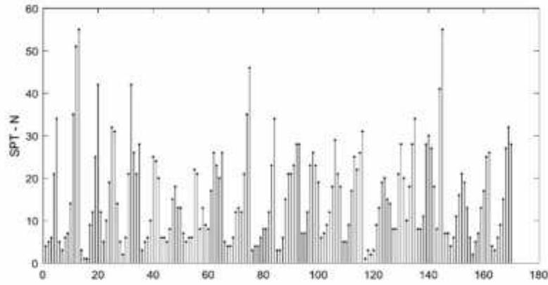
**Fig. 5.** SPT values of all the boreholes
