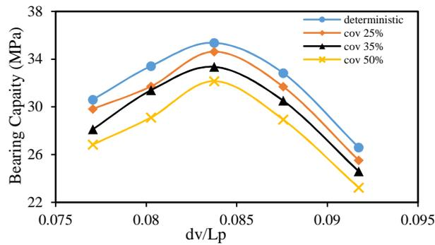
Fig. 7. Bearing capacity variation for pile diameter of 0.6m using Meyerhof 1956
