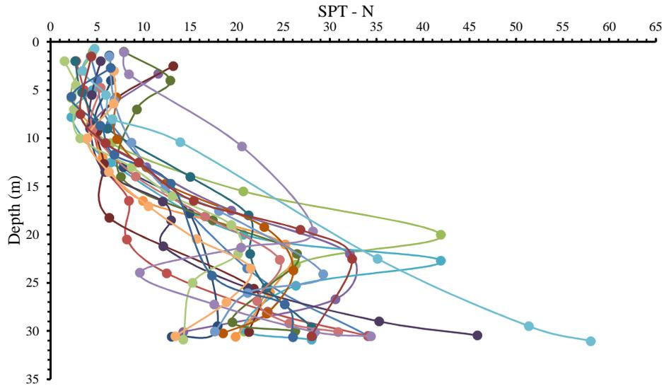
**Fig. 1.** SPT profiles for twenty borehole data
