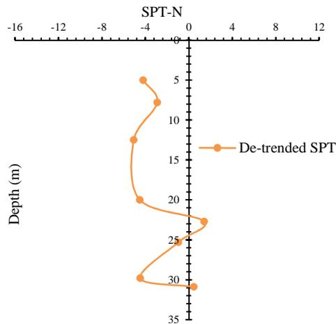
**Fig. 3.** De-trended SPT profile for the borehole-5
