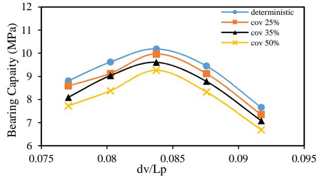
Fig. 11. Bearing capacity variation using Decourt 1995
