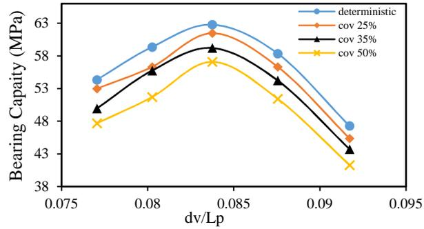
**Fig. 8.** Bearing capacity variation for pile diameter of 0.8m using Meyerhof 1956
