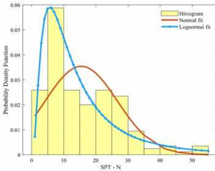
**Fig. 6.** Histogram and probabilistic distributional fit of SPT – N values
