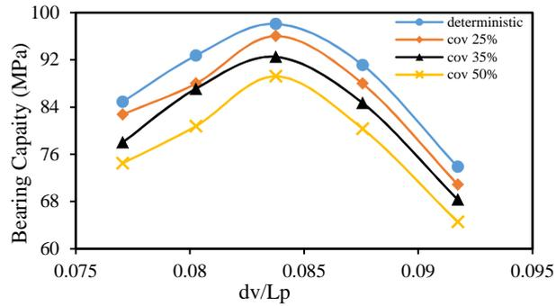
**Fig. 9.** Bearing capacity variation for pile diameter of 1.0 m using Meyerhof 1956
