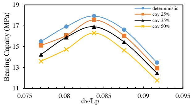
**Fig. 10.** Bearing capacity variation using Aoki and De'Alencar 1975
