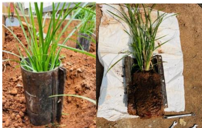
Fig.2. Sampling of specimen using split cylindrical sampler
