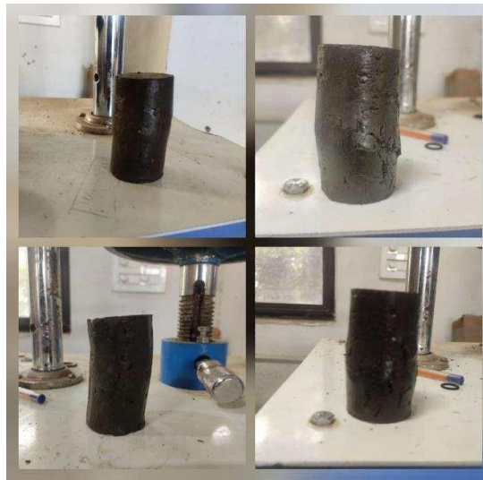
Fig. 2. Failure of soil sample
