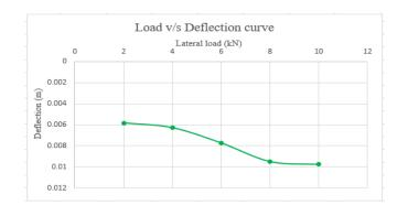
Fig 2. Load v/s deflection curve for pile without casing
