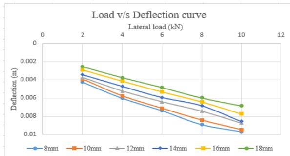
Fig 5. Load v/s deflection curve for pile with polypropylene casing
