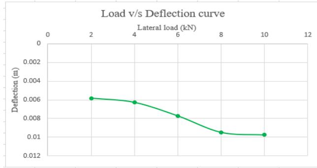
**Fig 2.** Load v/s deflection curve for pile without casing
