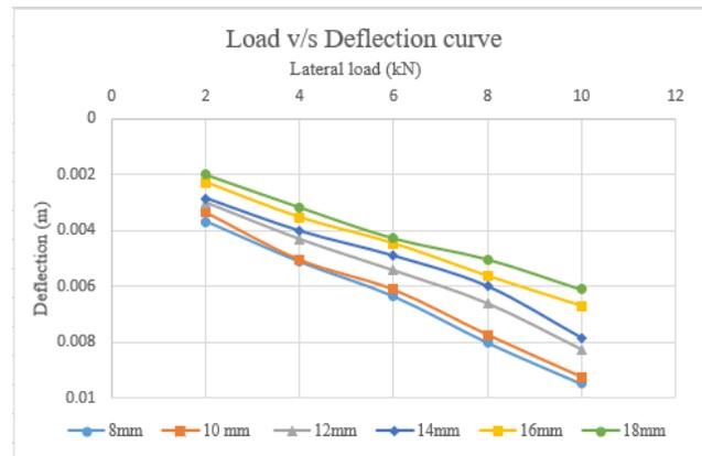
**Fig 3.** Load v/s deflection curve for pile with steel casing
