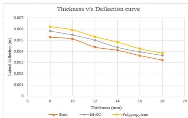
**Fig 1.** Thickness v/s lateral load curve for the design load
