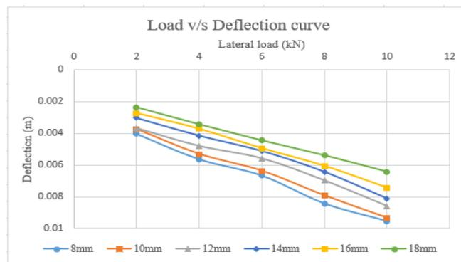
**Fig 4.** Load v/s deflection curve for pile with BFRC casing
