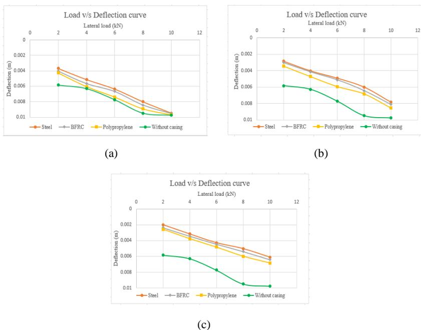
Fig 6. Load v/s deflection curve for pile with (a) 8mm (b) 14mm (c) 18mm casing
