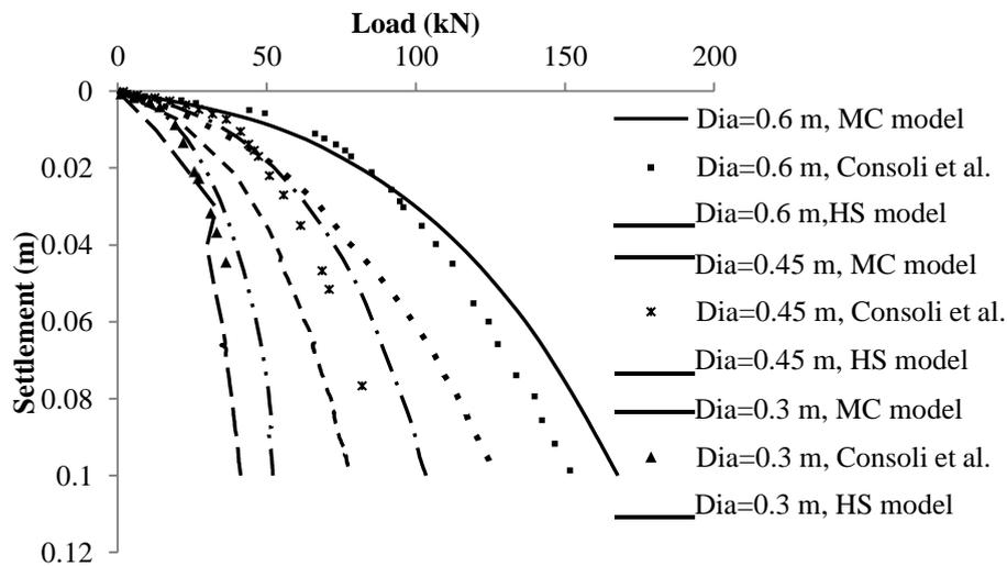
**Fig. 1.** Load settlement behavior of circular footing obtained from Consoli et al. (1998) and numerical models.
