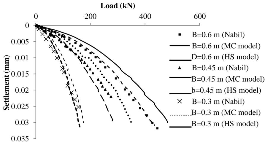
**Fig. 2.** Load settlement behavior of circular footing obtained from Nabil. (1996) and numerical models.
