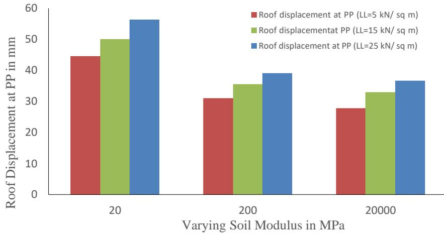
**Fig. 8.** Roof Displacement at Performance points with Varying Live Loads for soil moduli of  $E_s = 20\text{MPa}$ ,  $E_s = 200\text{MPa}$  and  $E_s = 20000\text{MPa}$ .
