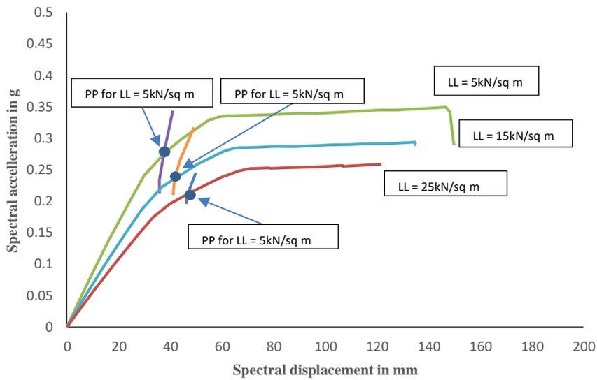
**Fig. 6.** Pushover curves and performance points with varying live loads in ADRS format for soil stiffness  $E_s = 20\text{MPa}$ .
