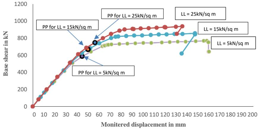
**Fig. 5.** Pushover curves and performance points with varying live loads for soil stiffness  $E_s = 20\text{MPa}$ .
