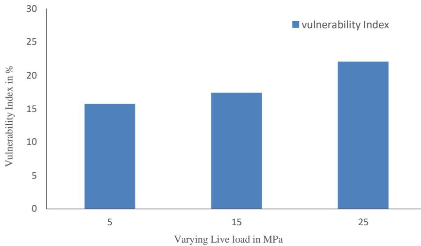
**Fig. 7.** Vulnerability Index with Varying Live Load for soil modulus  $E_s = 20$ MPa.
