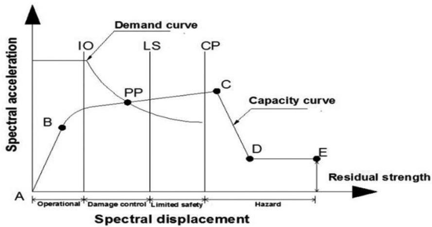
IO: Immediate Occupancy, LS: Life Safety, CP: Collapse Prevention, C: Collapse, PP: Performance Point.
