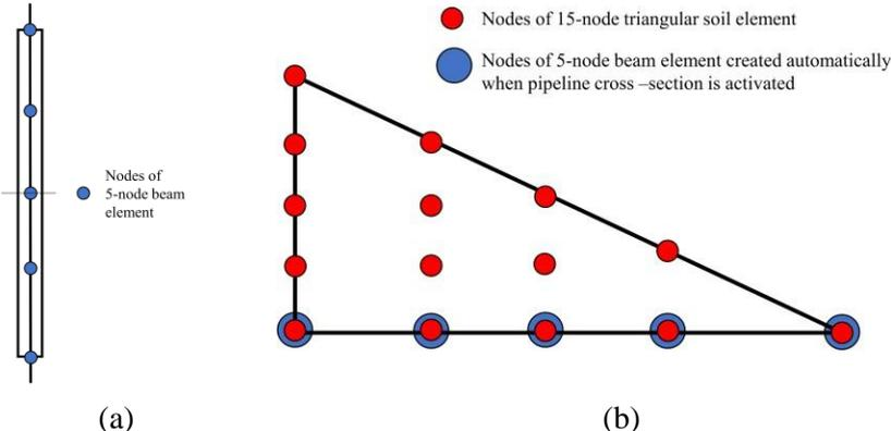
Figure 2: A typical diagram of a (a) 5-node beam element constituting the pipe cross-section and a (b) 15-node triangular element constituting the soil volume.
