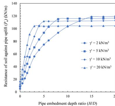
Figure 4. Variation of resistance against pipe uplift with pipe embedment depth ratio for homogeneous soil bed.
