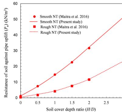
Figure 3. Comparison between the  $P_u$  predicted by the current model and the  $P_u$  obtained from the previous studies in the case of the weightless soil ( $\gamma' = 0$ )
