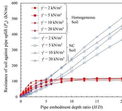
Figure 8. Comparison between resistance against pipe uplift within a homogeneous soil bed and a normally consolidated soil bed.
