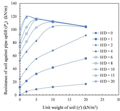
Figure 5. Variation of resistance against pipe uplift with a unit weight of soil for homogeneous soil bed.
