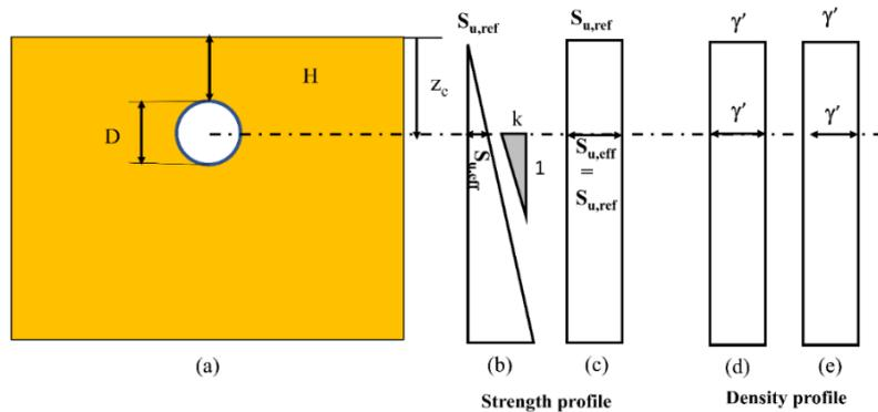
Figure 1. A visualization of the (a) schematic diagram of the pipe soil system; (b) and (c) strength profile for NC and homogeneous soil, respectively; and (d) and (e) density profile for NC and homogeneous soil, respectively.
