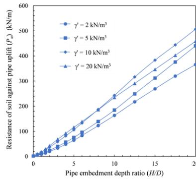
Figure 6. Variation of resistance against pipe uplift with pipe embedment depth ratio for normally consolidated soil bed.
