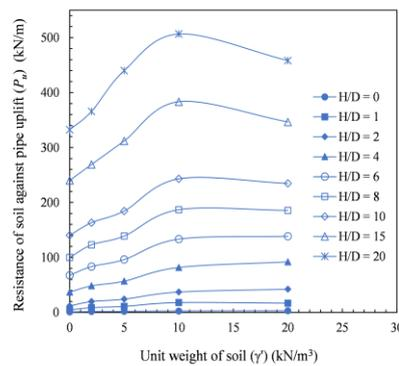
Figure 7. Variation of resistance against pipe uplift with a unit weight of soil for normally consolidated soil bed.
