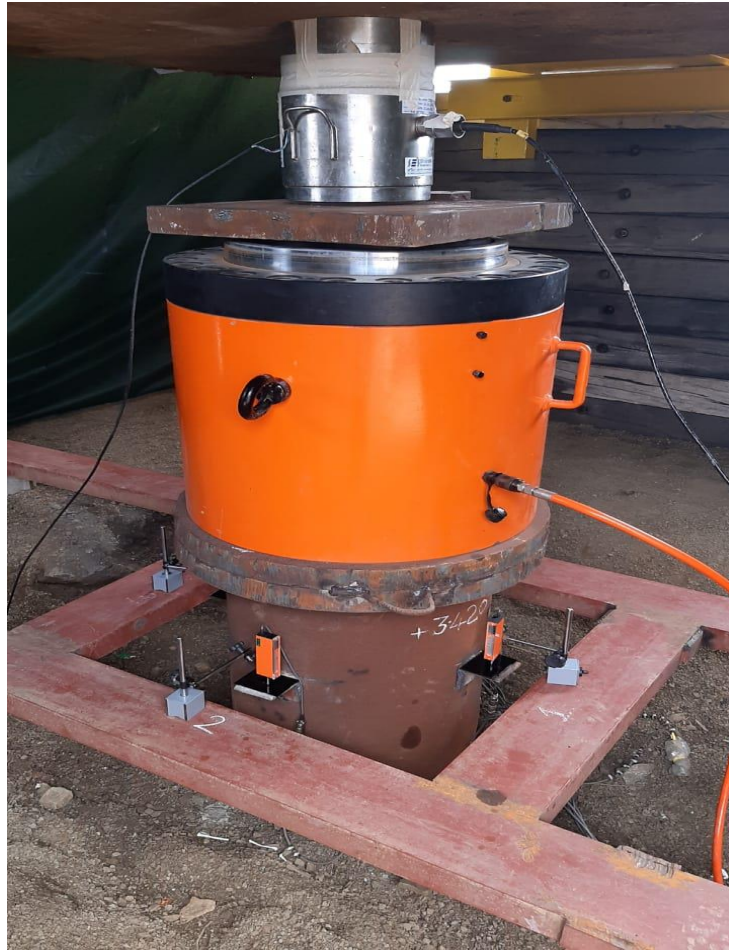
Fig.1. Typical set up for static load test
