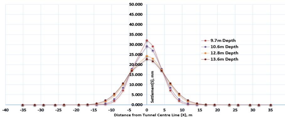
**Fig 9.** Comparison of Ground settlement for different tunnel depths at very stiff sandy clayey silt.
