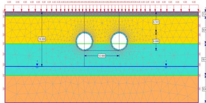
**Fig. 2.** Model view of geotechnical profile, tunnel cross section along with tunnel depth of 9.7m.
