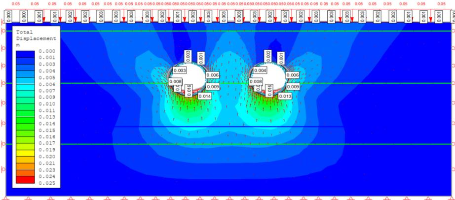
**Fig. 5.** Ground Settlement from numerical model (FEM) for tunnel depth of 9.7m.
