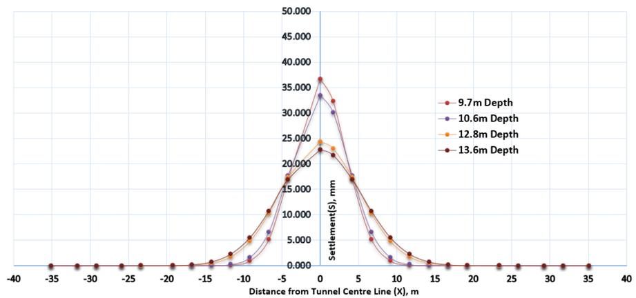
Fig.4. Comparison of surface settlement predicted by empirical method for different tunnel depth.
