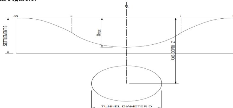
**Fig. 1.** Normal distribution curve (error function curve) to represent the cross-section of settlement trough.
