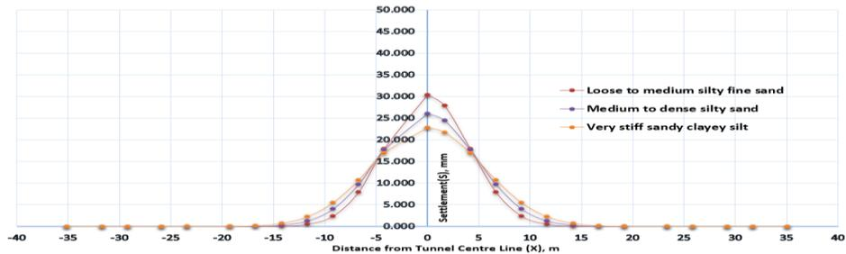
**Fig. 13:** Comparison of Ground settlement for 13.6m tunnel depth at 3 different ground conditions.
