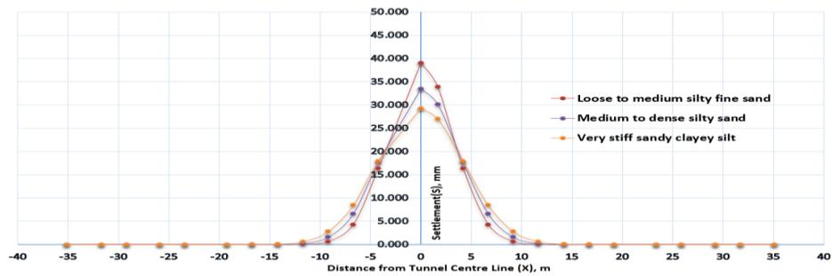
**Fig. 11.** Comparison of Ground settlement for 10.6m tunnel depth at 3 different ground conditions.
