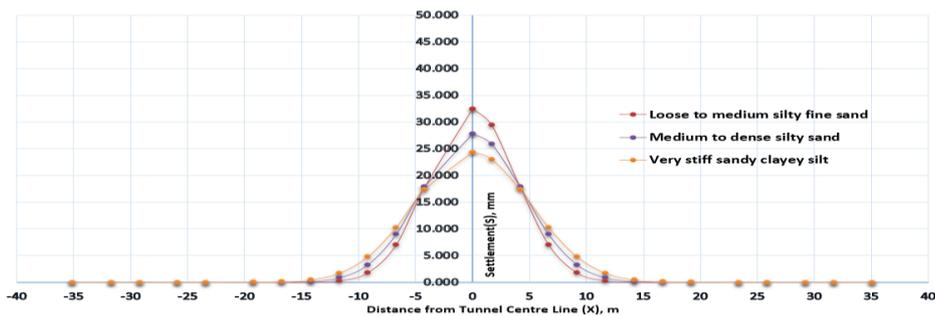
**Fig .12.** Comparison of Ground settlement for 12.8m tunnel depth at 3 different ground conditions.
