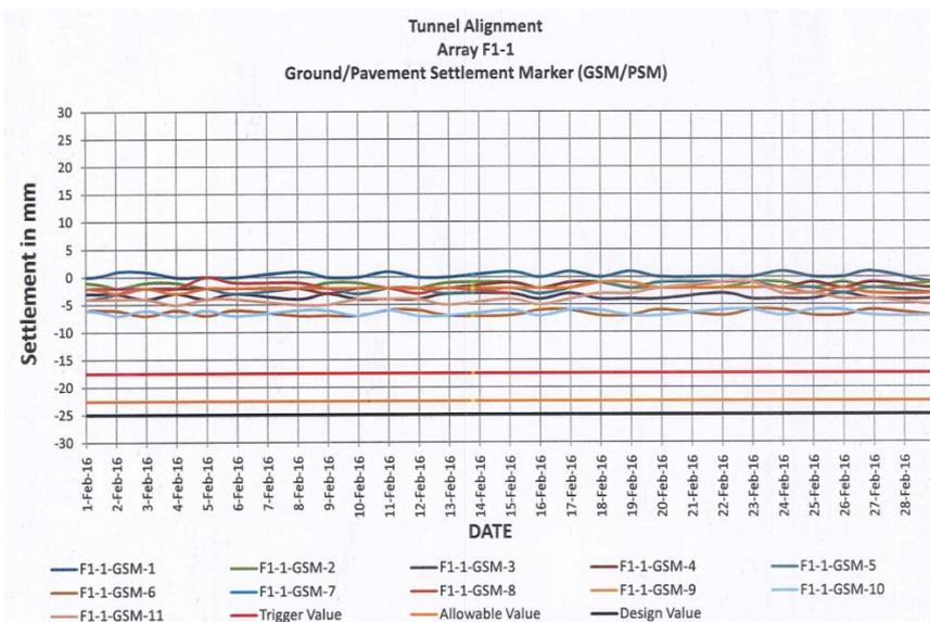
**Fig. 6.** Ground settlement data recorded at project site.
