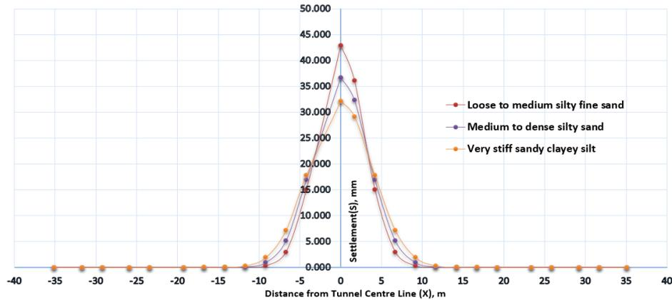
**Fig.10.** Comparison of Ground settlement for 9.7m tunnel depth at 3 different ground conditions.
