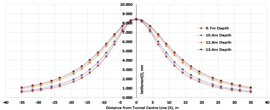
Fig. 3. Comparison of surface settlement predicted by analytical method (elasticity solution) for different tunnel depth.
