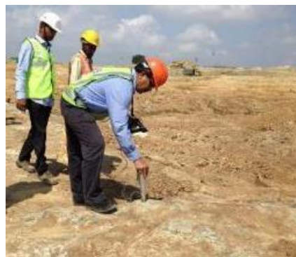
Fig. 2. Assessment of insitu strength of rock
