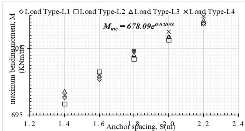
Fig. 4. Variation of maximum bending moment with anchor spacing in MC model
