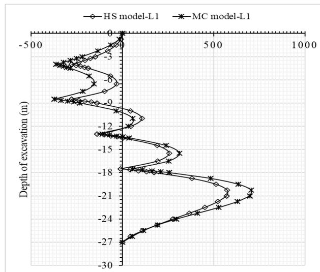
**Fig. 10.** Variation of bending moment with depth of excavation in both HS & MC model
