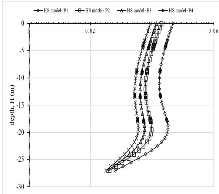
Fig. 7. Variation of horizontal wall deflection with depth and pre-stress force in HS model.
