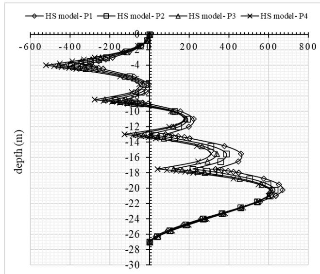
**Fig.9.** Variation of wall bending moment with depth and pre-stress force in HS model
