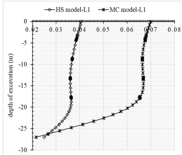
Fig. 11. Variation of lateral wall deflection with depth of excavation in both HS & MC model
