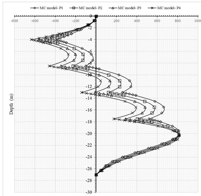
Fig.8. Variation of wall bending moment with depth and pre-stress force in MC model
