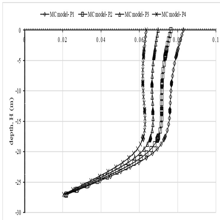
**Fig. 6.** Variation of horizontal wall deflection with depth and pre-stress force in MC model.
