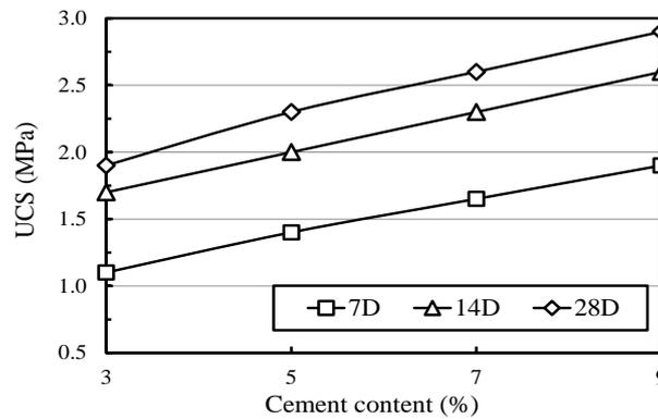
Fig. 2 Variation of UCS values of laterite-stone chips-cement mix with cement content
