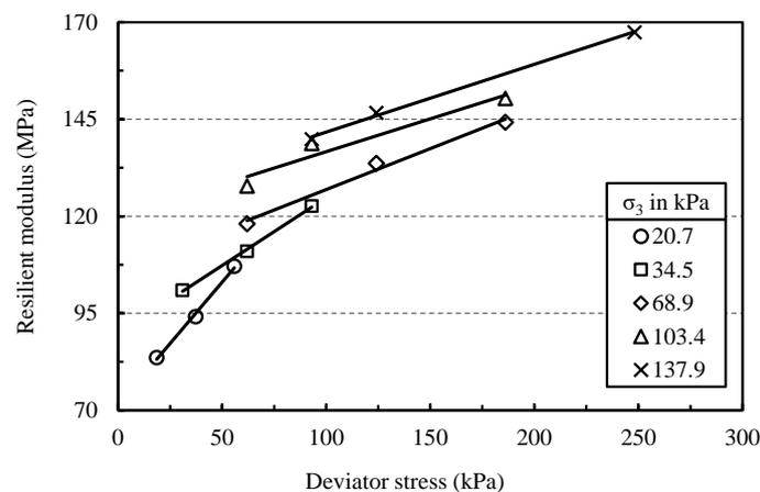
**Fig. 4** Effect of deviator stress and confining stress on resilient modulus of optimum LSC mix cured for 28 days
