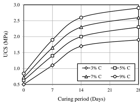
Fig. 3 Variation of UCS values of laterite-stone chips-cement mix with curing period
