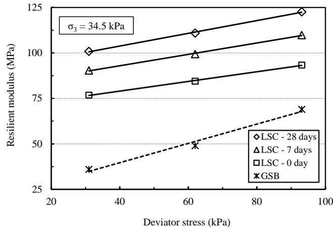
**Fig. 5** Comparison of resilient modulus of optimum LSC mix for various curing periods with GSB at a constant cell pressure of 34.5 kPa
