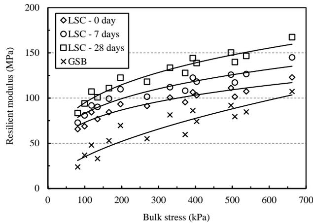
**Fig. 6**  $M_r$  vs bulk stress for LSC mixes and GSB
