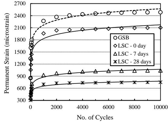
Fig. 7 Permanent strain of LSC mixes and GSB
