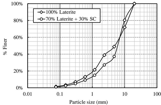
**Fig. 1** Particle size distribution curve for 100% laterite gravel and 70% laterite gravel + 30% stone chips
