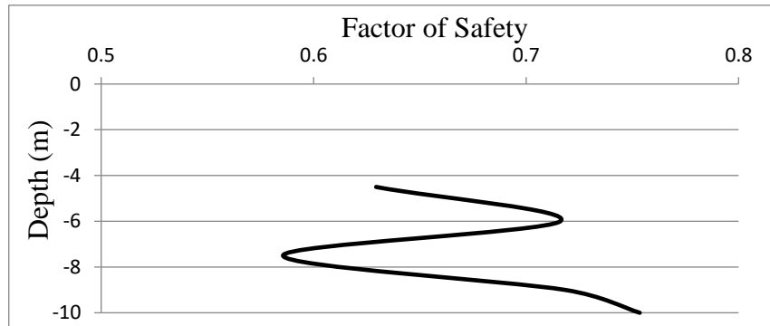
Fig. 3b. Factor of safety against the liquefaction
