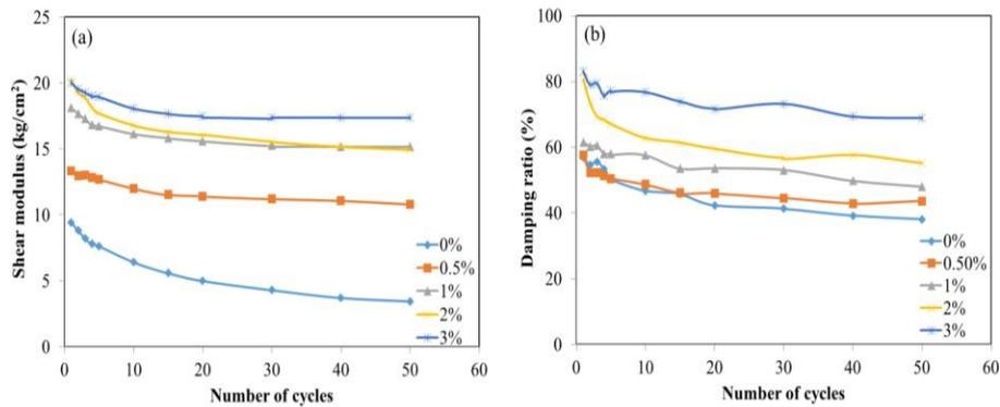
**Fig. 2.** Effect of biopolymer content on (a) secant shear modulus (b) damping ratio
