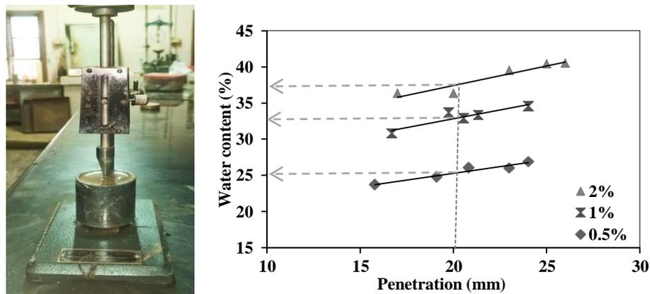
**Fig. 1.** (a) Cone penetrometer apparatus (b) Liquid limit of treated soil at different concentration of agar biopolymer using cone penetration test.
