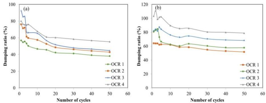
Fig. 5. Effect of OCR on damping ratio of (a) untreated soil and (b) 2% agar treated soil
