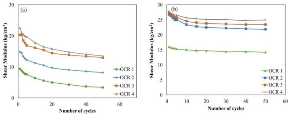
Fig. 4. Effect of OCR on secant shear modulus of (a) untreated soil and (b) 2% agar treated soil
