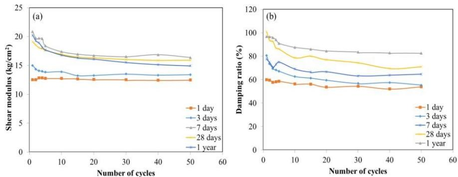
**Fig. 3.** Effect of curing period on (a) secant shear modulus (b) damping ratio
