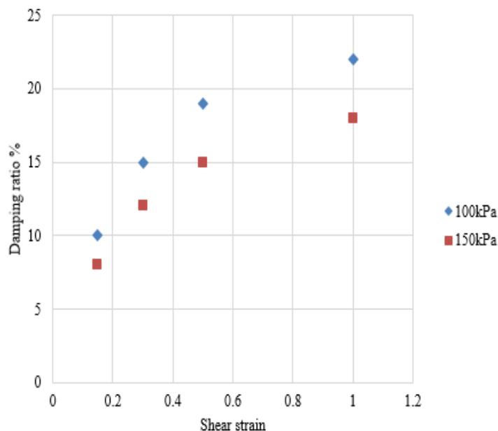
**Fig.5.** shear strain effect on damping ratio of clayey sand at relative density 70%
