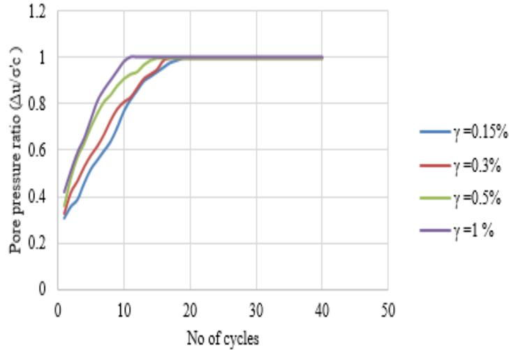
**Fig.3.** Shear strain effect on pore water pressure ratio ( $r_u$ ) of clayey sand at relative density 70%.
