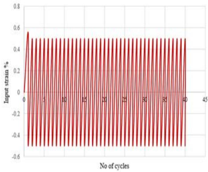
**Fig.2.1 (a):** Shear strain vs. No. of loading cycles.
