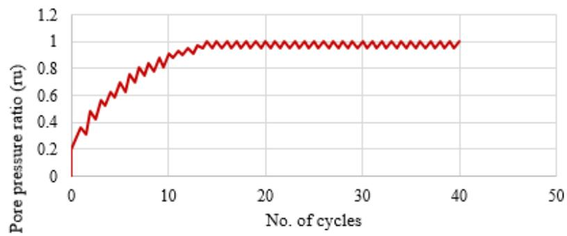
Fig.2.2(c): Pore water pressure ratio vs No. of cycles.
