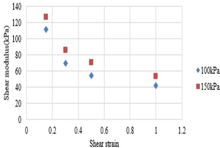
**Fig.4.** Shear strain effect on shear modulus of clayey sand at relative density 70%
