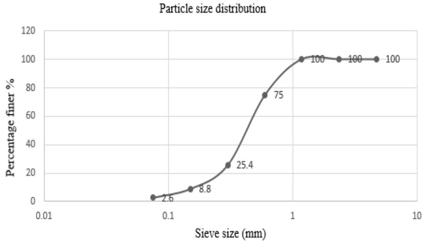
Fig. 1. Particle size distribution of sand
