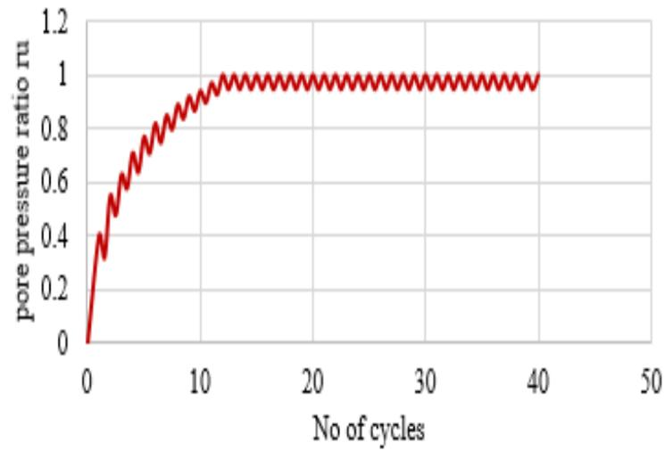
**Fig.2.1(c):** Pore water pressure ratio vs. No. of cycles.
