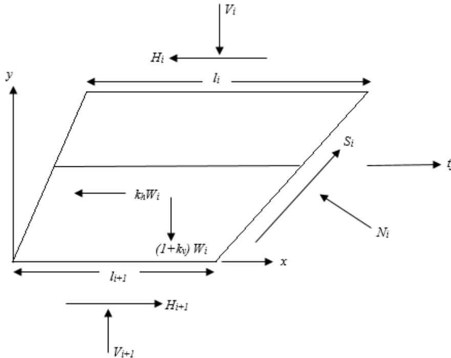
**Fig. 1.** Forces acting on single horizontal slice with reinforcement.
