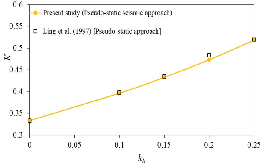
**Fig. 2.** Comparison of non-dimensional total required tensile strength from the deterministic analysis
