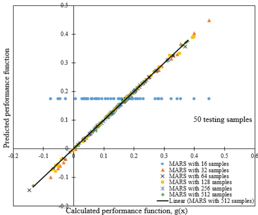
**Fig. 3.** Comparison between the values of performance function predicted by MARS models and the ones calculated by LEM
