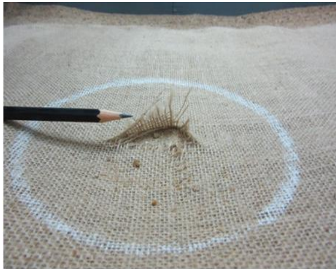
Fig. 4. Image of ruptured jute geotextile after plate load test.
