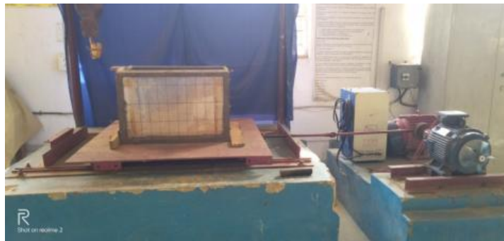
Fig. 1. Arrangement of the shake table Instrument
