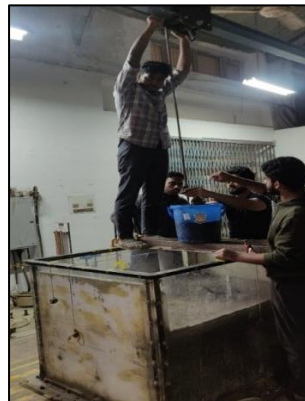
Fig. 4. Filling of geotextile tube
