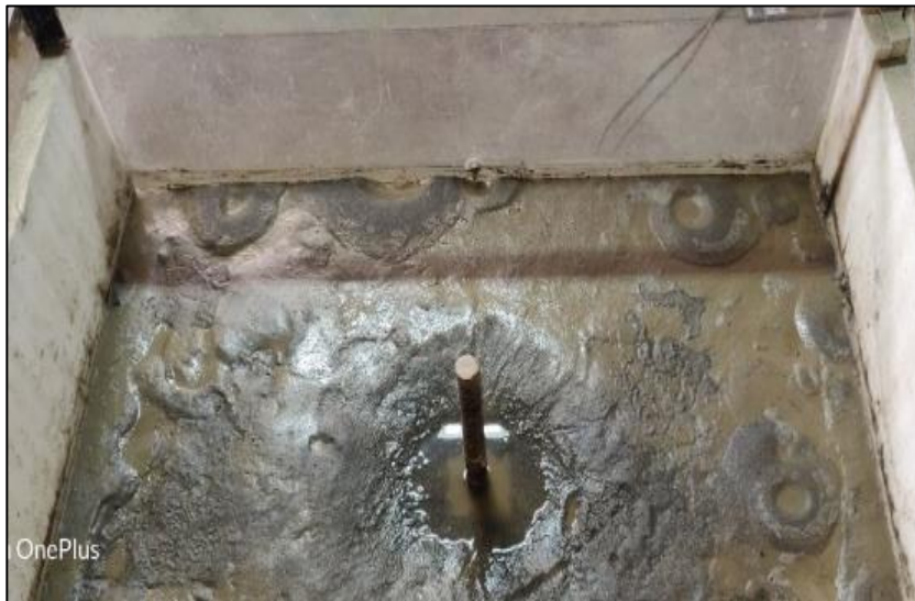
Fig. 7. Formation of sand boils after 0.3g acceleration (Unreinforced condition)
