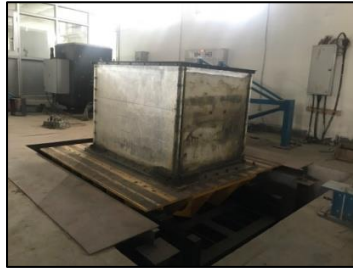
Fig. 1. Perspex glass tank placed over shaking table
