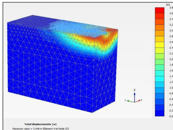
**Fig. 6.** Total displacements of original soil stratum.
