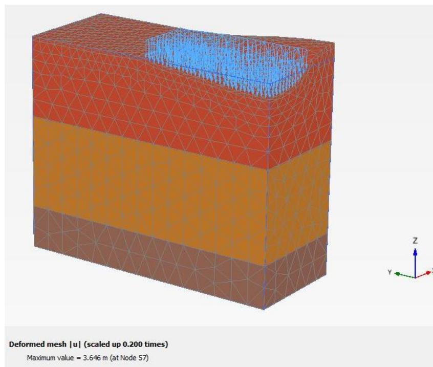
**Fig. 8.** Deformed mesh of Original soil stratum
