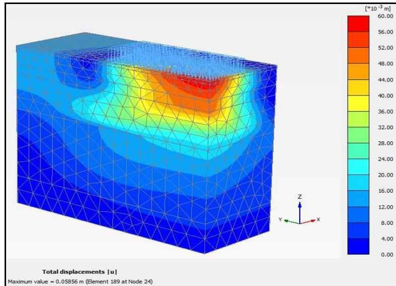
**Fig. 7.** Total predicted displacements of reinforced soil stratum.
