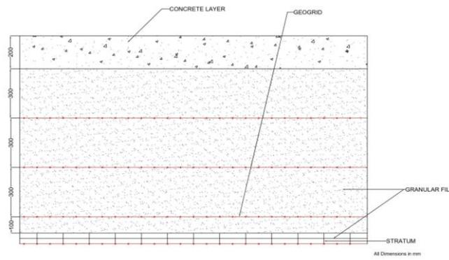
**Fig. 5a.** Layout of Reinforced soil stratum of thickness 1.65 m includes MSL, geogrid and cellular mattress.
