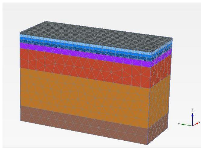
**Fig. 5b.** FEA mesh of Reinforced soil stratum
