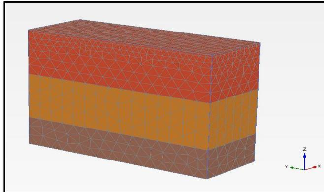
**Fig. 4.** FEA mesh of original soil stratum
