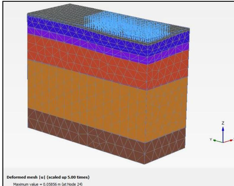
**Fig. 9.** Deformed mesh of reinforced soil stratum
