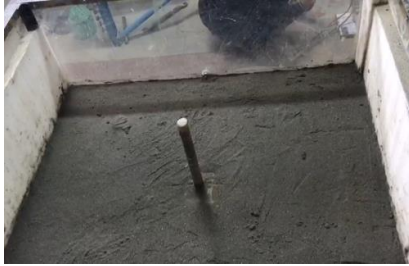
Fig. 2. Unreinforced bed – 40% RD – Initial condition
