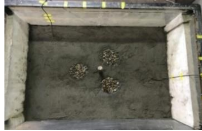
Fig. 3. SC reinforced bed – 40% RD – Initial condition
