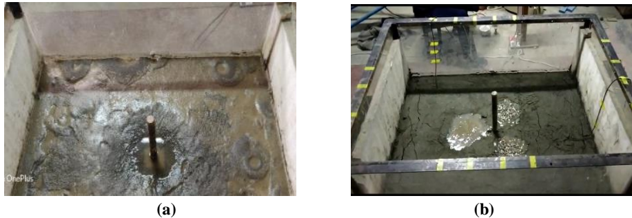
Fig. 5. (a) Sand boils depicting generation of EPWP in unreinforced bed (b) Water seeping out initially from the gravel drains in SC reinforced bed.
