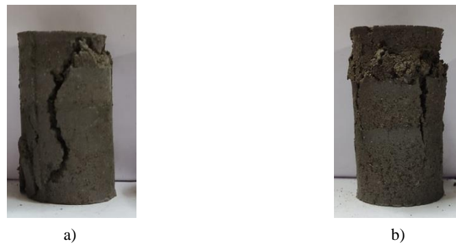
Fig. 6. Failure pattern observed in a) Heat curing b) Moist curing
