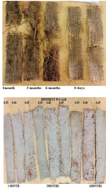
Fig. 6. Soil burial images of untreated and treated jute after 1, 3 and 6 months.
