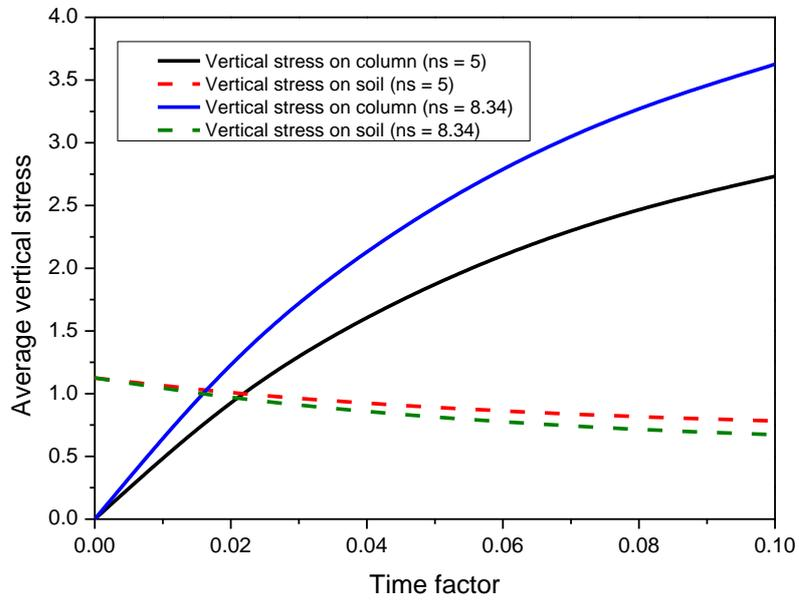
Fig. 2. Variation of average vertical stress with Time factor
