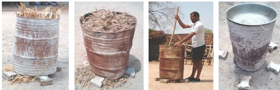
Fig.3. Drums are filled with crop residues, compacted and covered with top lid after lit on fire at bottom and left for sometime so that pyrolysis takes place.
