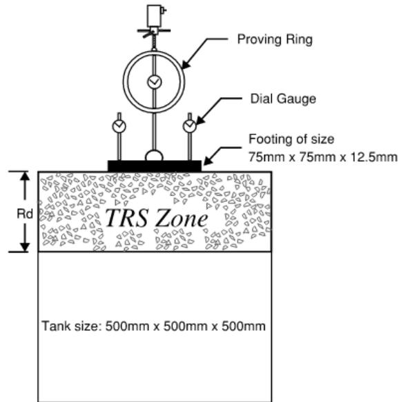
**Fig. 3.** Schematic diagram of the test setup
