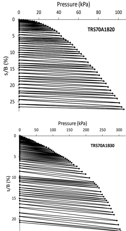
Fig. 5. Pressure settlement curve of reinforced sand
