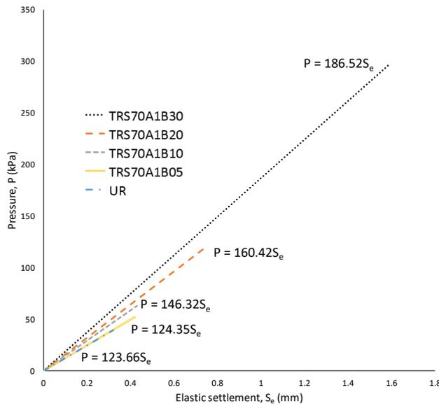
Fig. 8. Pressure v/s Elastic Settlement curve at different tire chip content
