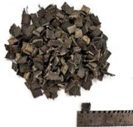
**Fig. 1.** Tire chips used in the experimental study
