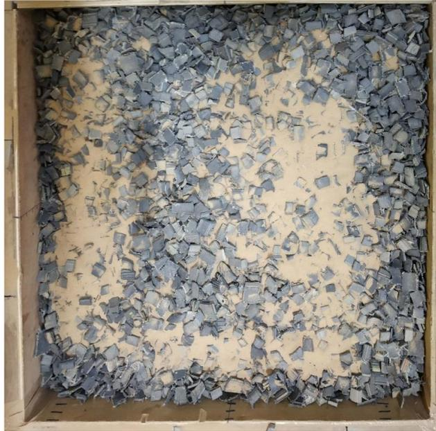
**Fig. 6.** Tire Chip reinforced sand (Sample: TRS70A1B40)
