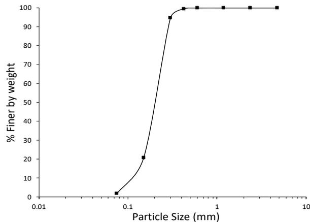
**Fig. 2.** Grain Size Distribution Curve of Local Sand
