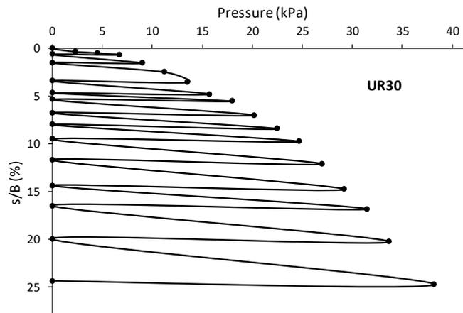
**Fig. 4.** Pressure settlement curve of unreinforced sand ( $D_r = 30\%$ )
