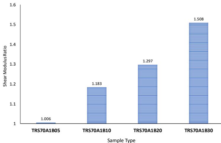
**Fig. 9.** Comparison of Shear modulus at different tire chip content
