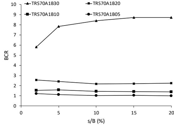
Fig. 7. Comparison of BCR at different tire chip content
