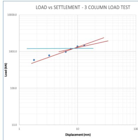
**Fig. 20.** Log-log Curve for Three Column Load Test
