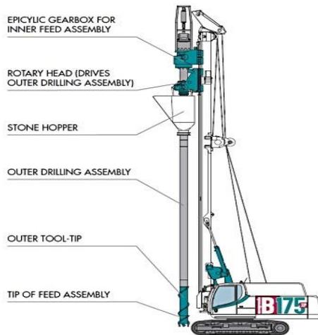
**Fig. 6.** Assembly for Non-Vibration Stone Column
