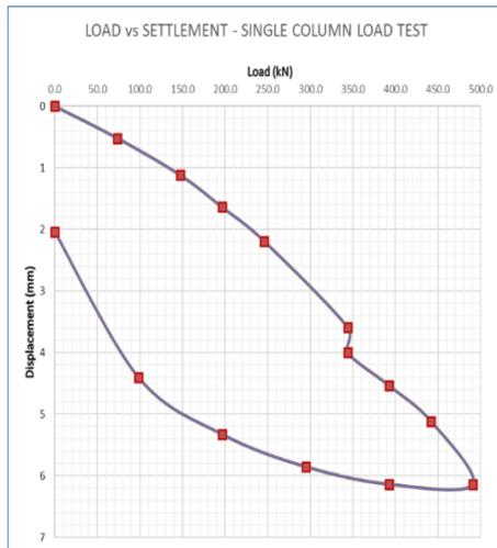
**Fig. 14.** Load Settlement Curve for Single Column Load Test
