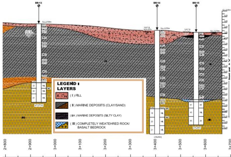
Fig. 1. Profile at DFCCIL Chainage from 2.800km to 3.700 km in JNPT area
