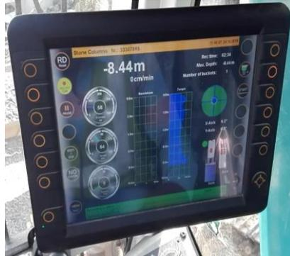
**Fig. 10.** Torque applied during initial boring of column
