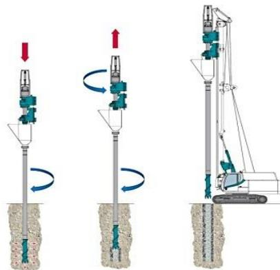
**Fig. 9.** Process of Installation of Stone Column
