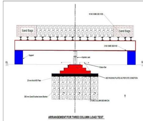
**Fig. 18.** Test Arrangement for Three-Column Load Test
