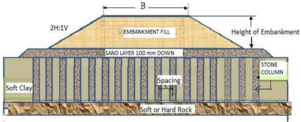
**Fig. 3.** Typical section of layout of stone column
