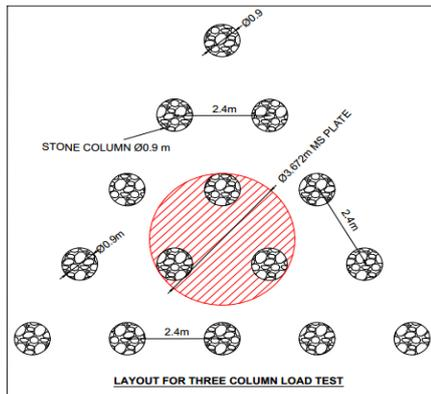
**Fig. 17.** Layout for Three Column Load Test
