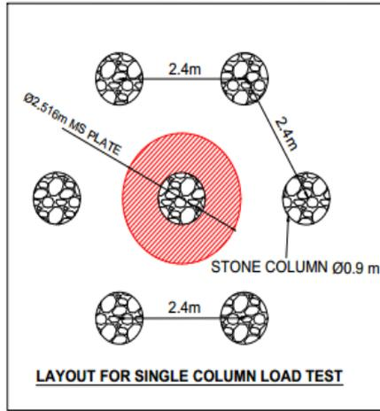
**Fig. 12.** Layout for Single Column Load Test
