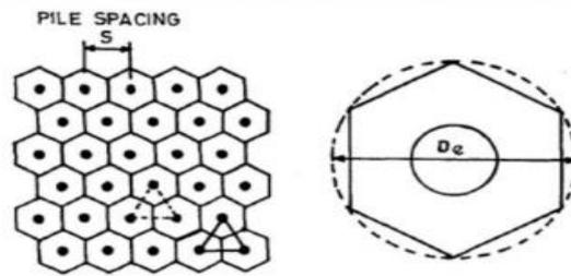
**Fig. 2.** Triangular pattern of stone column
