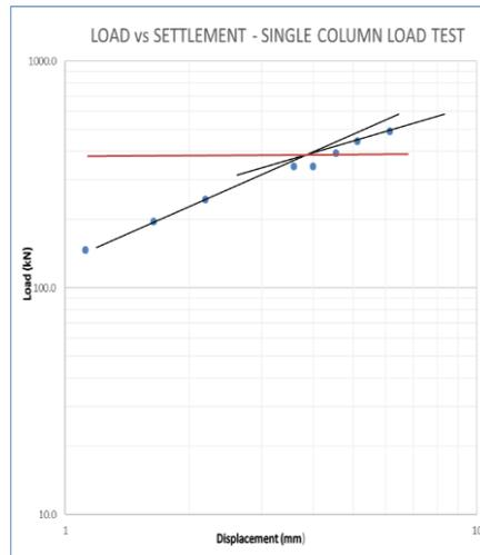
**Fig. 15.** Log-log Curve for Single Column Load Test
