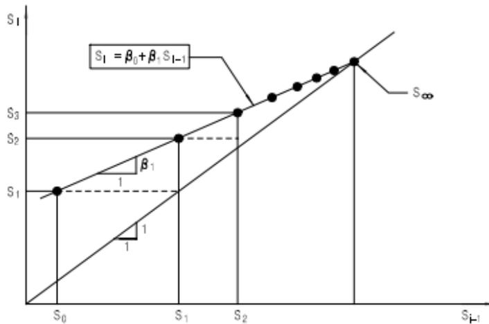
**Fig. 4.** Asaoka's Graphical Method of Settlement prediction
