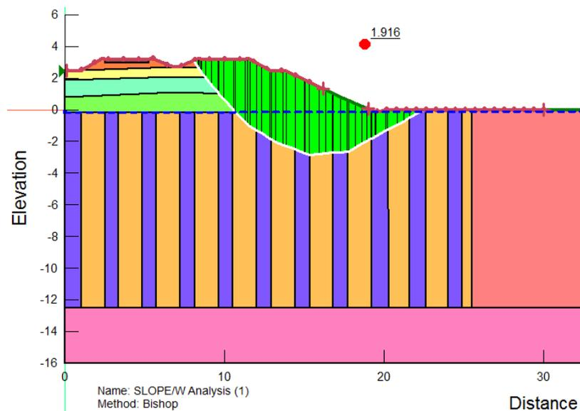
**Fig. 5.** Stability Analysis of Embankment with Stone Column Reinforcement
