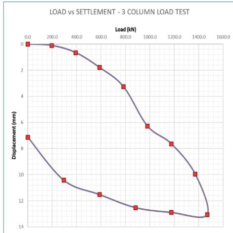
**Fig. 19.** Load Settlement Curve for Three Column Load Test
