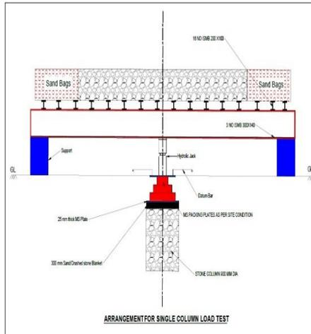
**Fig. 13.** Test Arrangement for Single-Column Load Test
