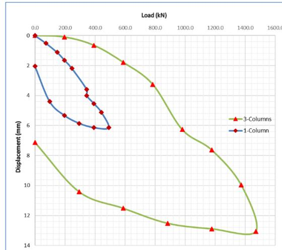
**Fig. 21.** Load Settlement Curves Comparison
