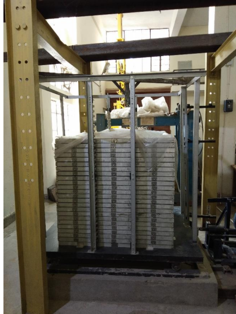
Fig. 1. Developed facility of shaking table with laminar box
