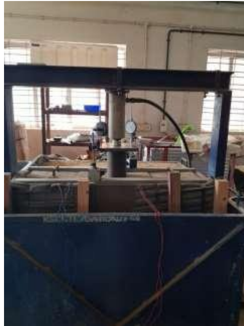
Fig. 2. Lateral Supports Provided for the Wall
