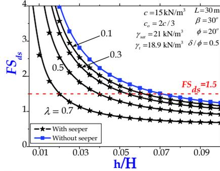
Fig. 8. Influence of the ratio of cover soil layer thickness to the height of landfill on  $FS_{ds}$ .
