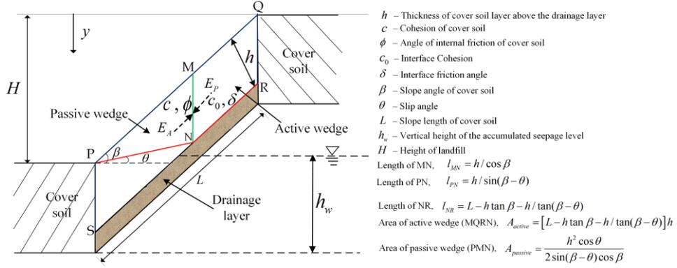
Fig. 2. Direct slip (*ds*) failure in veneer cover soil in the presence of internal seepers.
