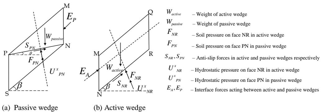
**Fig. 4.** Stress analysis diagrams of active and passive wedges when there is an internal seeper.
