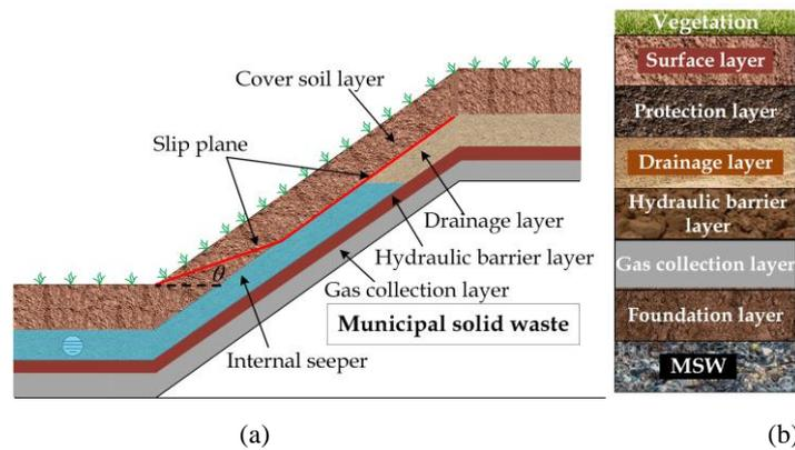
**Fig. 1.** (a) Internal seep in the drainage layer of veneer cover system, (b) Components of veneer cover system
