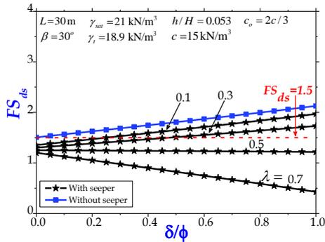
Fig. 10. Influence of the ratio of interface friction angle to cover soil friction angle on  $FS_{ds}$ .
