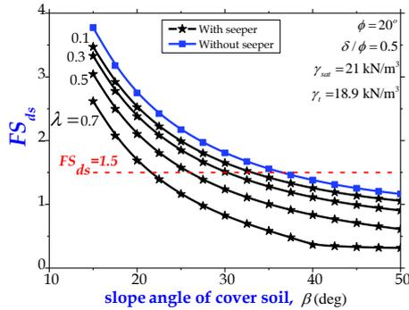
Fig. 7. Influence of slope angle on  $FS_{ds}$ .
