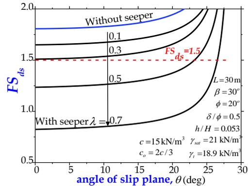
**Fig. 6.** Effect of slip angle on  $FS_{ds}$ .
