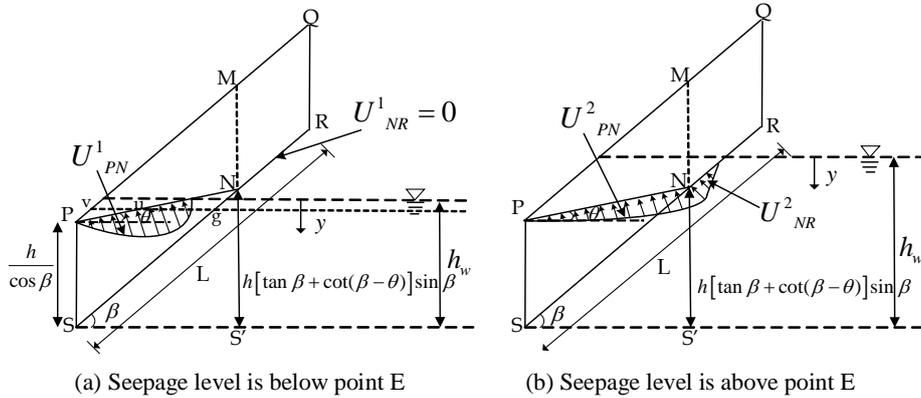
**Fig. 3.** Computation models for  $ds$  failure in veneer cover soil with the presence of internal seepers under two different conditions.
