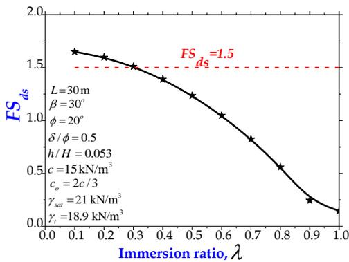
**Fig. 5.** Effect of immersion ratio on  $FS_{ds}$  in the presence of internal seeper.
