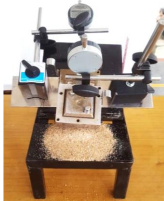
Fig.4. Failure of sand sample under gravity
