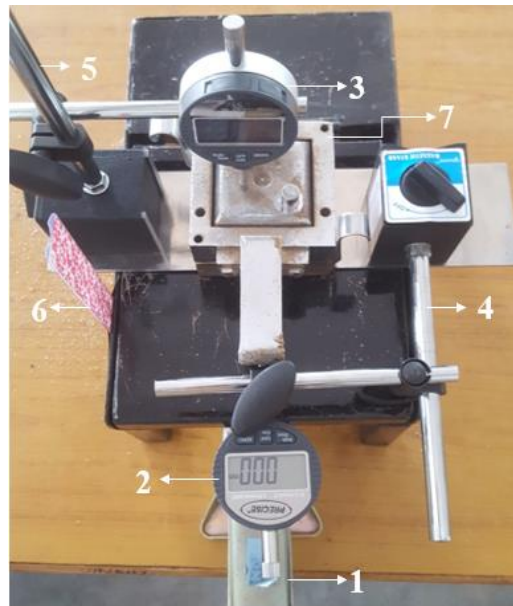
Fig.1. Gravity Induced shear test set-up (1)Lifting jack, (2)Dial gauge (to measure horizontal displacement), (3)Dial gauge (to measure dilation), (4 &5)Magnetic stands(6)Graduation scale,(7) Shear box (6 cm x 6 cm)
