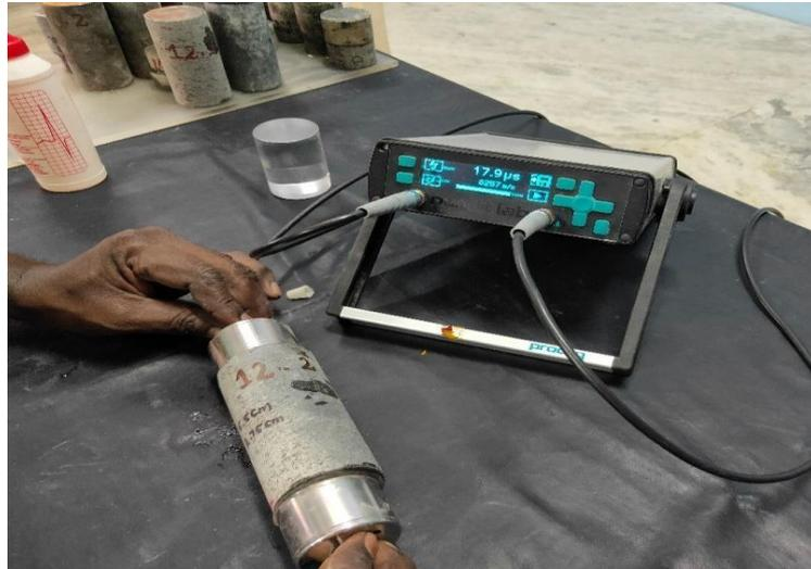
**Fig. 2. UPV test on a core specimen**
