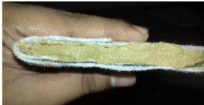
Fig.4. GCL prepared using dredge material and 40 % bentonite
