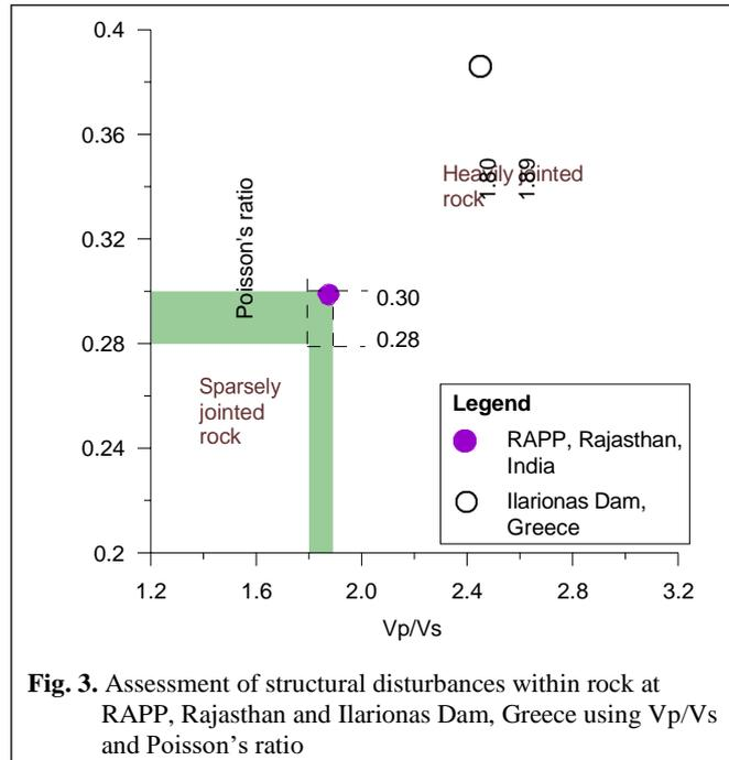
**Fig. 3.** Assessment of structural disturbances within rock at RAPP, Rajasthan and Ilarionas Dam, Greece using  $V_p/V_s$  and Poisson's ratio
