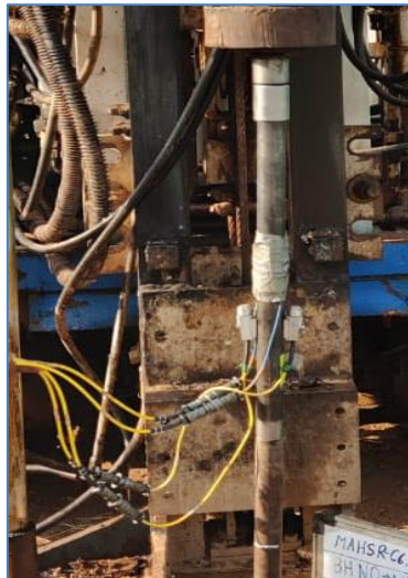
Fig 3. ETR Test Set-up
