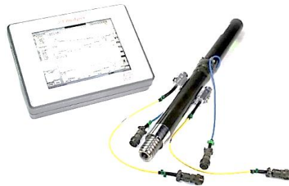
Fig 2. Instrumented AW rod and Data Acquisition System
