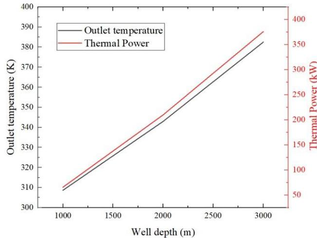
**Fig. 6.** Variation of outlet fluid temperature and thermal power with well depth
