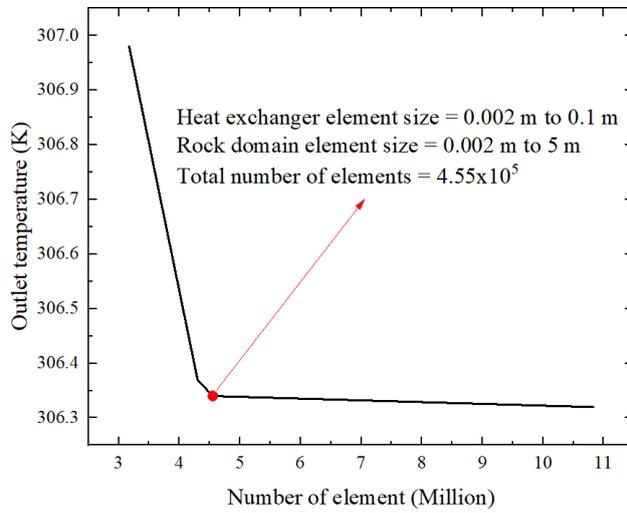
**Fig. 4.** Grid independence study for 1000 m length CBHE
