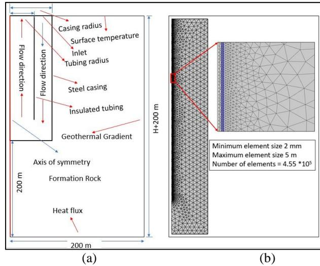
**Fig. 3.** Numerical modelling (a) Axisymmetric model domain (b) Triangular elemental mesh
