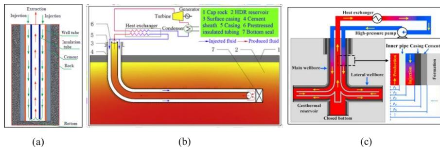
**Fig. 2.** HDR reservoir with CDHE (a) Vertical well [6] (b) Horizontal well [30] (c) Multi-lateral wells [31]
