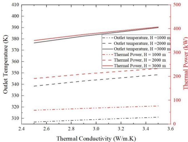
**Fig. 8.** Variation of outlet fluid temperature and thermal power with rock thermal conductivity
