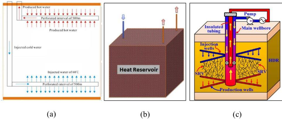
**Fig. 1.** (a) Two horizontal wells EGS [25] (b) Triplet with triangular pattern [26] (c) Multi-lateral well system [27]
