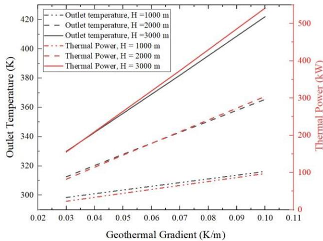
**Fig. 7.** Variation of outlet fluid temperature and thermal power with geothermal gradient
