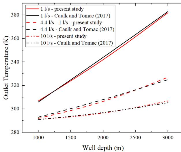
**Fig. 5.** Borehole heat exchanger outlet temperature for various well depths, mass flow rates at 0.07 K/m
