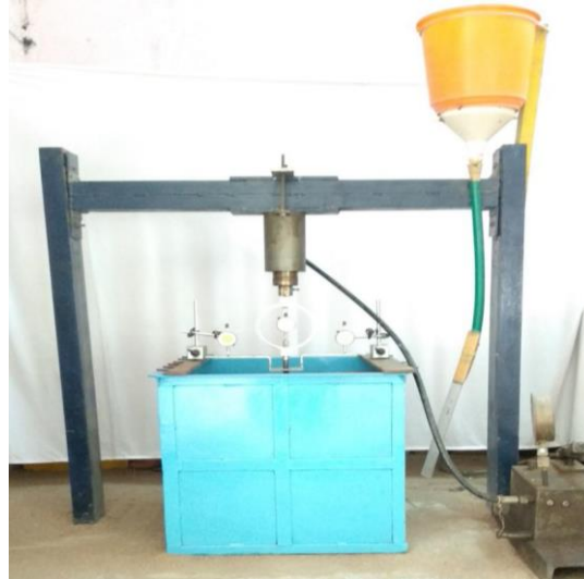
Fig.1. Test setup used for vertical loading on Helical piles
