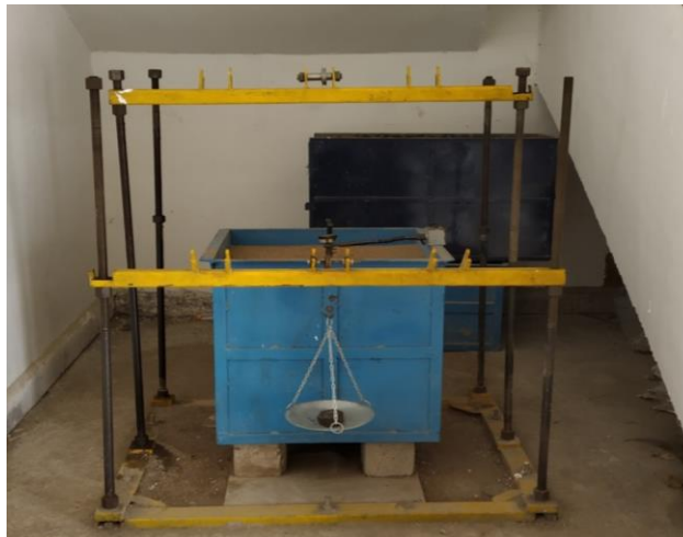
Fig. 2. Test setup for lateral loading on Helical pile
