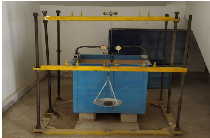
Fig. 3. Test setup for uplift loading on Helical pile
