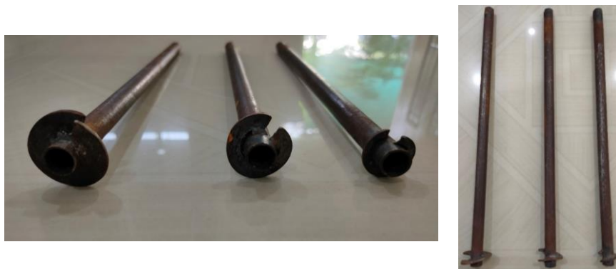
Fig. 4. Model helical pile used in experimental investigation
