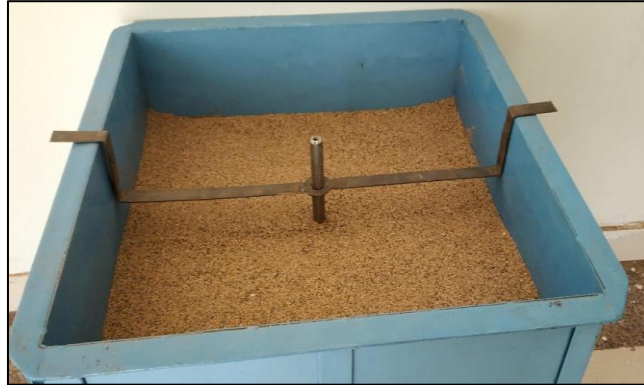
Fig. 3. Undisturbed Method of Pile Installation During Experimental Investigations
