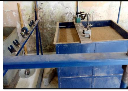
Experimental Setup used for Lateral Loading
