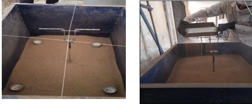
Fig. 3. Preparation of sand bed using rainfall techniques
