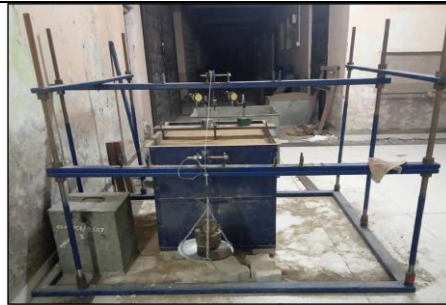
Experimental Setup used for uplift Loading
