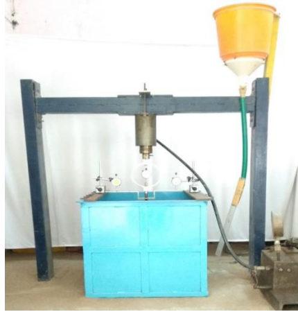
Fig. 1. Test setup used for vertical loading on Barrette piles
