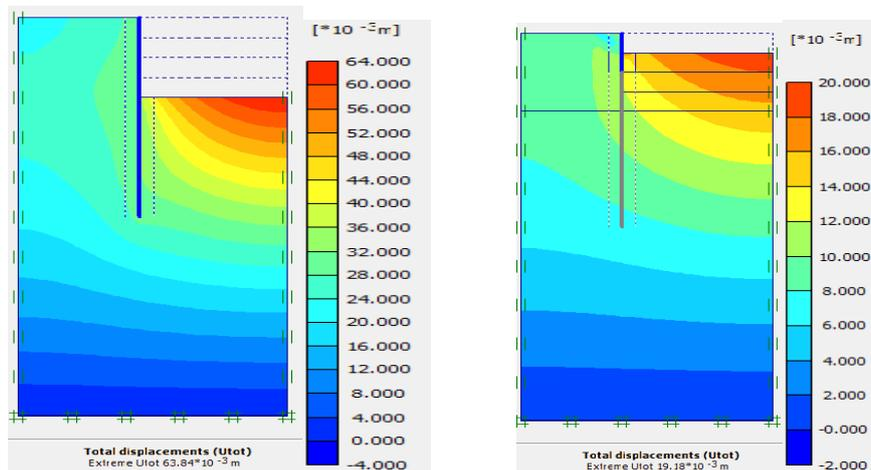
Fig.13. Displacement Contour for Unjointed Pile and Jointed Pile
