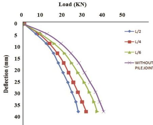
**Fig. 9.** Lateral Load Deflection Curve in Stiff Clay for various joint locations
