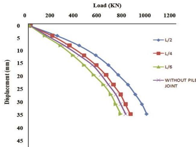
**Fig .10.** Combined Load Deflection Curve in Medium Sand for various joint locations
