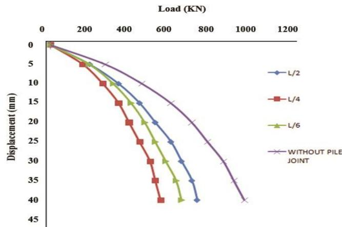
**Fig.11.** Combined Load Deflection Curve in Stiff Clay for various joint locations
