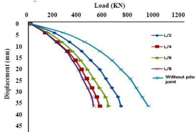
**Fig.6.** Load Settlement Response for various Joint Position in Stiff Clay
