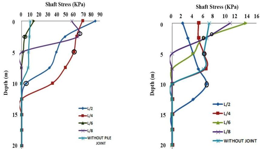
Fig.7. Shaft Stress Distribution Curve in Medium Sand and Stiff Clay
