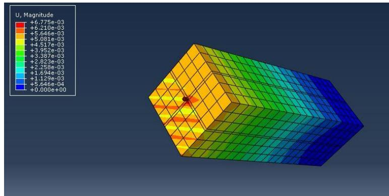
Fig.4. Displacement Contour for Jointed Pile
