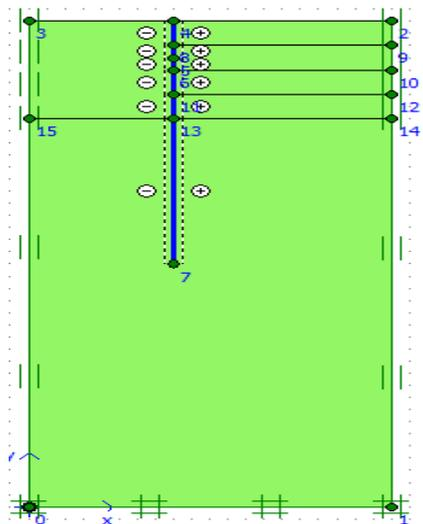
**Fig. 3. (a)** Model Excavation of Jointed Pile
