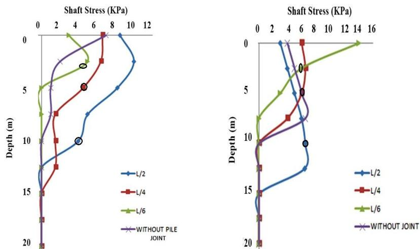
**Fig.12..** Shaft Stress Distribution Curve in Medium Sand and Stiff Clay-Variou s joint
