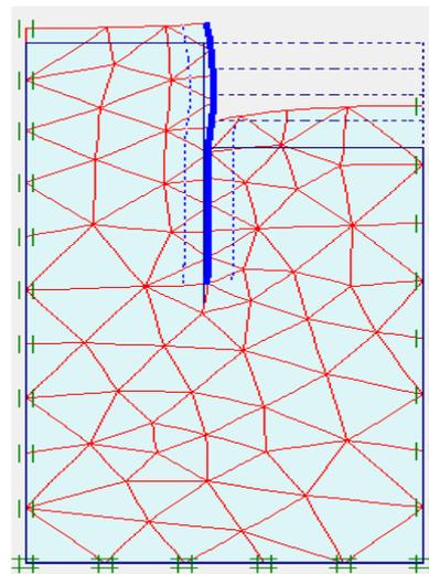
**Fig. 3. (b)** Deformed Mesh PLAXIS 2D
