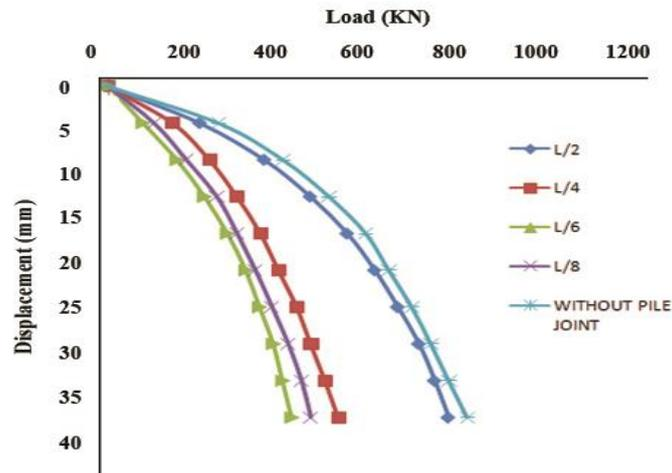
Fig. 5. Load Settlement Response for various Joint Position in Medium sand
