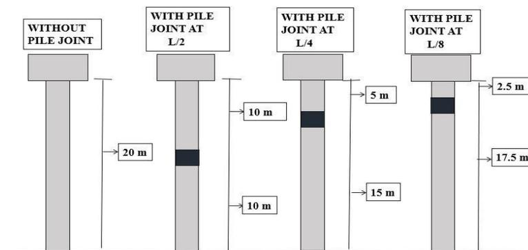
Fig. 1. Pile Joint Layout
