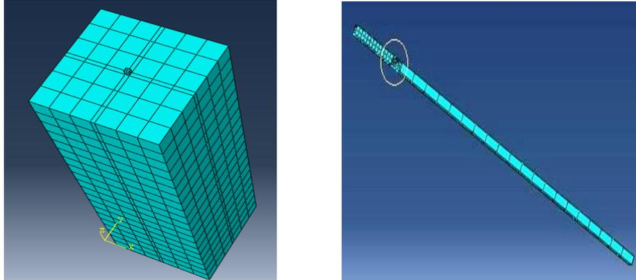
**Fig. 2.** Finite Element Mesh for Soil Mass and Jointed Piles
