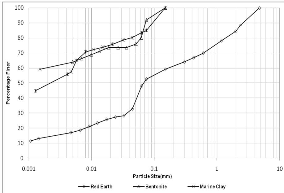
**Fig.2.** Grain Size distribution curves of Red Earth, Bentonite and Marine Clay
