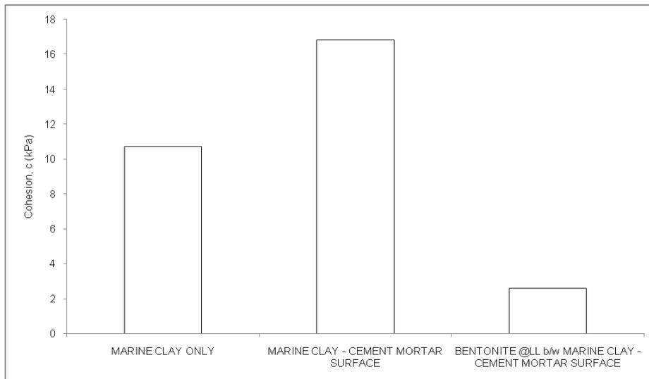
**Fig. 5.** Effect of type of interface on cohesion.
