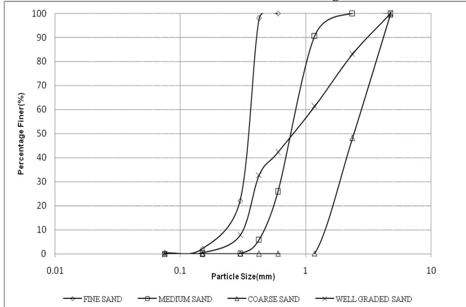
**Fig.1.** Grain size distribution curves of different fractions of sand
