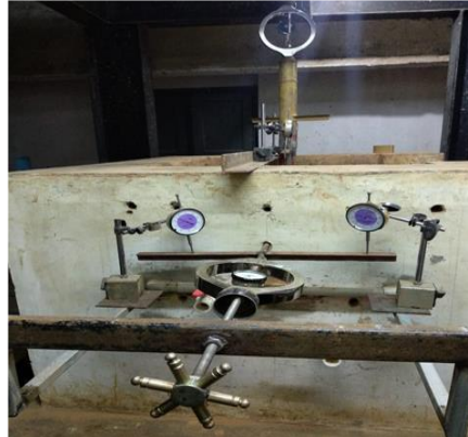
Fig. 4. Arrangement for lateral loading
